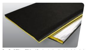
SuperDuct® RC is an FSK-faced fiberglass duct board insulation designed to be fabricated into rectangular ducts. Each board comes with a male or female shiplap to help make the fabrication process more efficient and accurate. The insulation itself has a glass mat airstream surface that is coated with the antimicrobial Permacote coating to improve durability and offer resistance to microbial growth.
