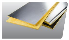
Mat-Faced Micro-Aire® is an FSK-faced fiberglass duct board insulation designed to be fabricated into rectangular ducts. The insulation features a glass mat airstream surface and male and female shiplaps to improve durability and efficiency during the fabrication process.
