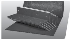
Linacoustic® RC-HP insulation is a flexible, fiberglass duct liner with higher density and enhanced acoustical control when compared to standard duct liners. The airstream surface is protected with JM's exclusive reinforced coating system, a glass mat surface coated with Permacote antimicrobial coating.
