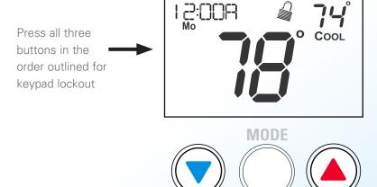
To *unlock* the keypad, press and hold the **MODE** button. While holding the **MODE** button, press the **WARMER** and **COOLER** buttons together, for five seconds. The icon will disappear from the display, then release the buttons.
