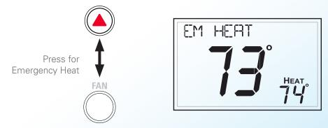
During Emergency Heat operation the thermostat will turn on the fan and the Aux strip heat (if installed) when there is a demand for heat. Also during Emergency Heat, heatpump operation will be unavailable.
