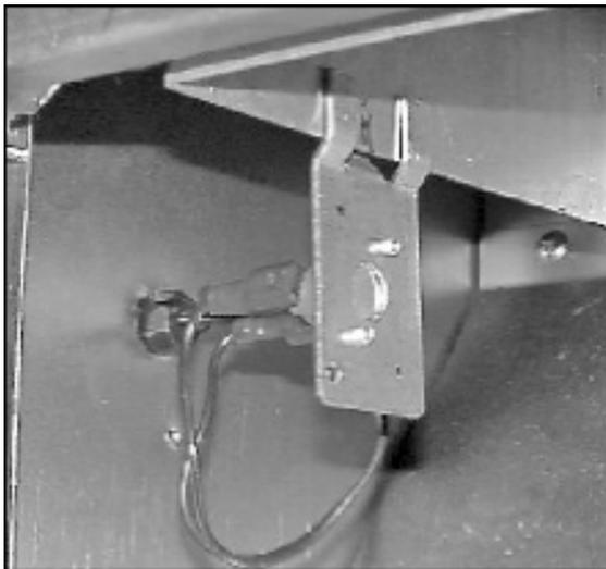
**Figure 4: Blocked Vent Switch**
