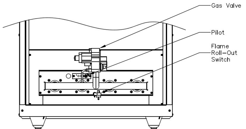
**Figure 5: Burner Compartment Area with Radiation Shield Omitted**
