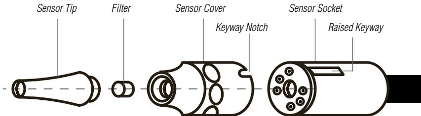
*To install sensor cover: align notch with raised keyway and insert straight on (do not twist)*
