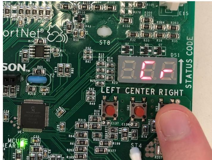
Then press “CENTER” to select the Cr menu. Some codes will begin flashing on the display. Ignore these codes and hold down the “LEFT” and “RIGHT” buttons simultaneously for at least 10 seconds. If the display switches to “Cr” again, check that the **Bluetooth®** Shared Data Loader is inserted fully into the connector and is powered on.
