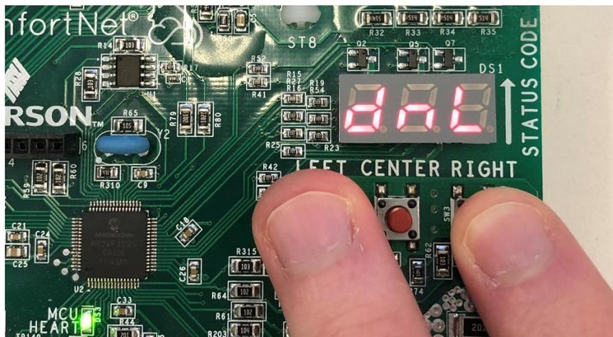
After holding “LEFT” and “RIGHT” for 10 seconds, the display will start flashing a new code (“dnL”), once this new code appears, release the “LEFT” and “RIGHT” buttons. The equipment
