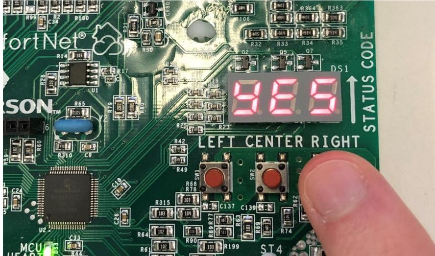
Then press the “CENTER” button **twice** to confirm the selection. The board will then start the Shared Data loading process. Once the Shared Data Loading process is complete, the display will return to displaying “Cr”.
