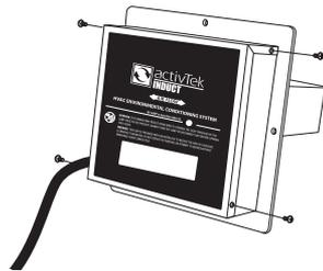
2. Open the cover of the unit by removing the four (4) thumb screws then remove the cover.
