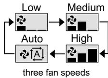
\* Auto cannot be selected if the indoor unit does not have Auto Fan speed function.
