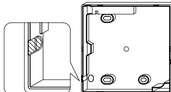
Cut the plastic at the notched area and remove any remaining burrs.
