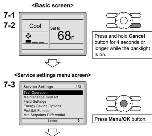
**7-4** Press **On/Off** button within 10 seconds, and the test operation starts. Monitor the operation of the indoor unit for a minimum of 10 minutes. During test operation, the indoor unit will continue to cool regardless of the temperature setpoint and room temperature.
