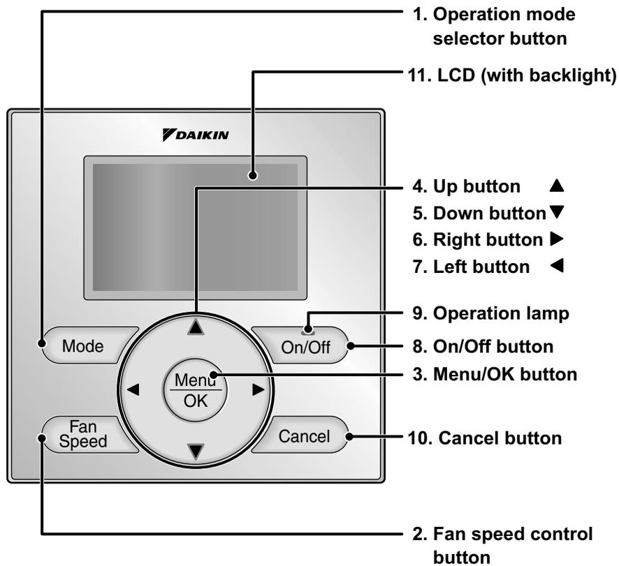
Functions other than basic operation items (i.e., On/Off, Operation Mode, Fan Speed, and Setpoint) are set from the menu screen.
