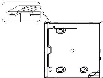
Cut the plastic at the notched area and remove any remaining burrs.
