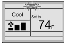
• Press **Mode** button several times until the desired mode Cool, Heat, Fan, or Auto mode is selected.
