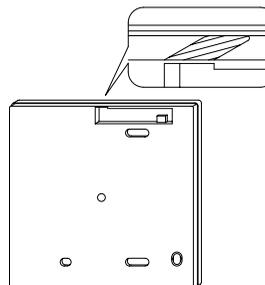
Cut the plastic at the notched area and remove any remaining burrs.
