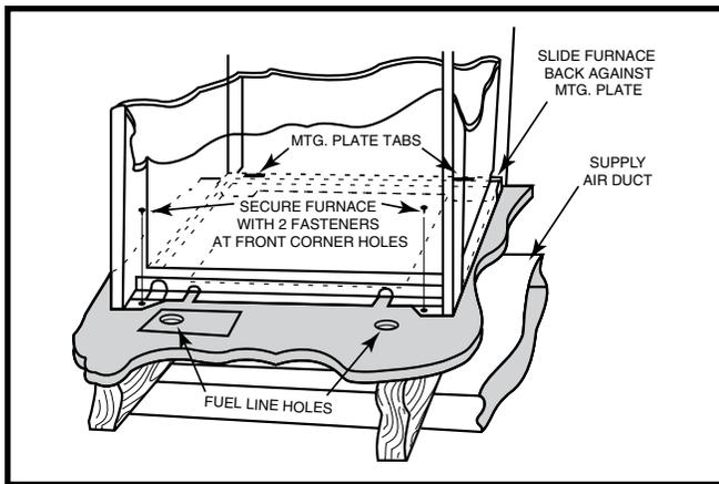
Figure 15. "A" Cabinet Furnace on Coil Cabinet
