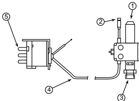
2. The automatic pilot must be mounted near enough to the main gas burner so it is easily ignited by the pilot ignition flame even when the pilot flame is reduced to the point where it is just sufficient to keep the pilot switch contacts closed.
