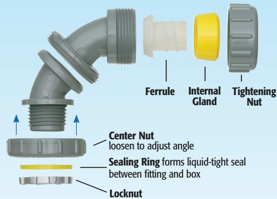
Arlington's no-spin ferrule allows the Zero to 90 connector to be secured to the conduit while fully assembled. To install, simply loosen the tightening nut and screw onto conduit. A positive liquid-tight seal is formed by the pressure sensitive internal gland as the nut is tightened. The sealing ring assures a liquid-tight seal between the fitting and box.
