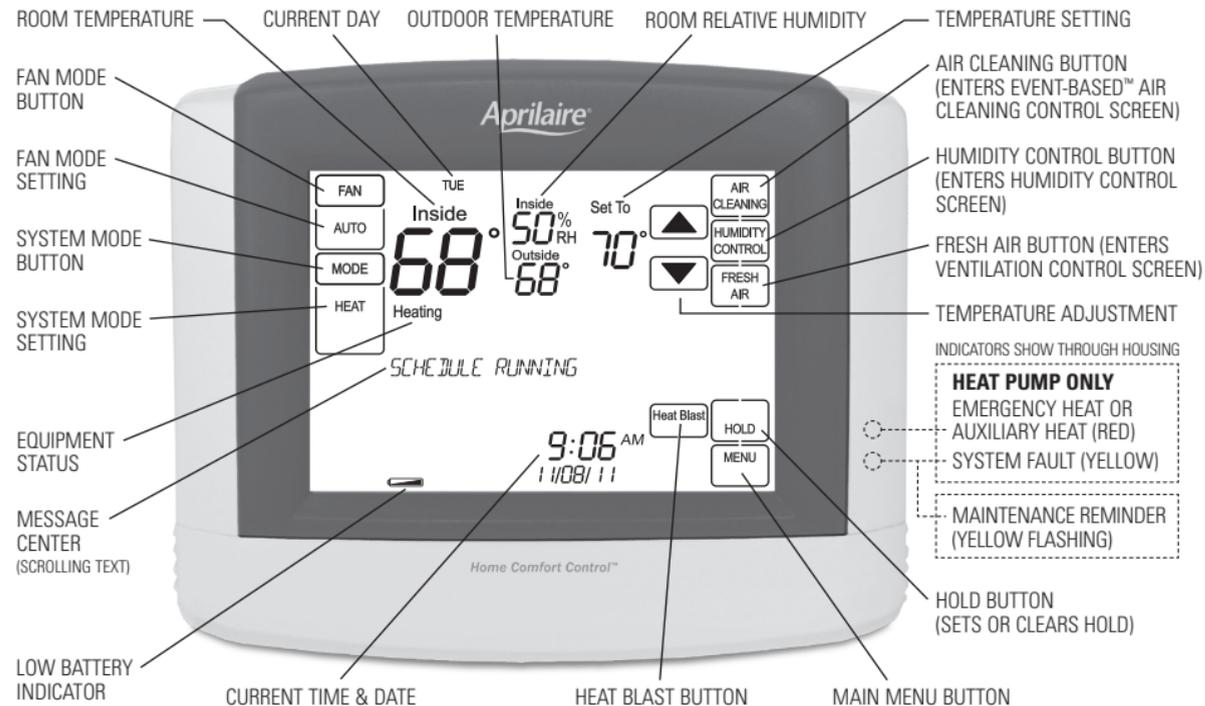
**NOTE:** BACKLIGHT IS ACTIVATED WITH FIRST BUTTON PRESS AND AUTOMATICALLY TURNS OFF.
