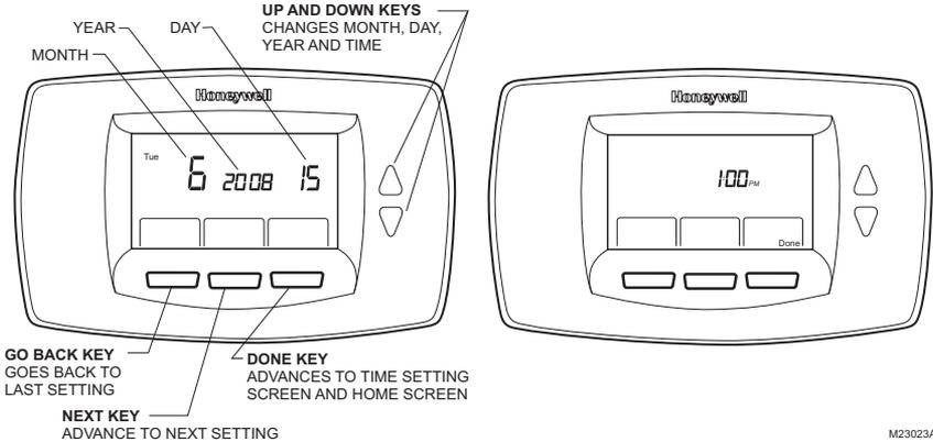
Fig. 25. Setting calendar and time after initial powerup.
