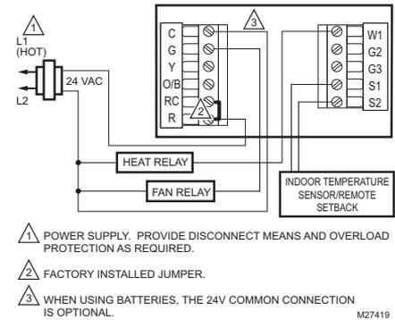
**Fig. 9. Typical hookup of heat-only system with fan.**
