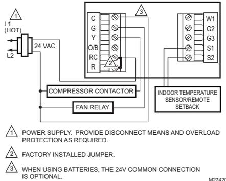
**Fig. 10. Typical hookup of cool-only system.**
