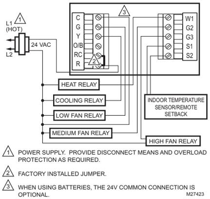
**Fig. 13. Typical wiring of 4 pipe fan coil.**
