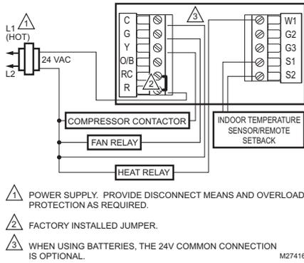
**Fig. 6. Typical wiring of single transformer 1H/1C system.**
