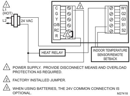
**Fig. 8. Typical hookup of heat-only system.**
