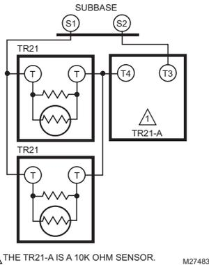
**Fig. 20. Wiring two TR21 (20K ohm) Sensors and one TR21-A (10K ohm) Sensor to provide a temperature averaging network**
