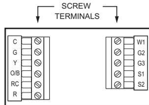
Fig. 4. Terminal identifications for system type.
