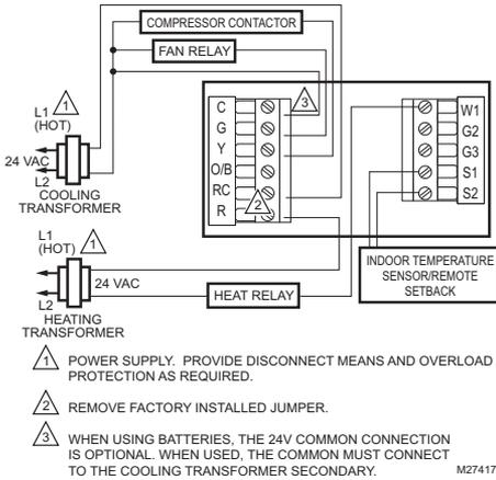
**Fig. 7. Typical hookup of dual transformer 1H/1C system.**
