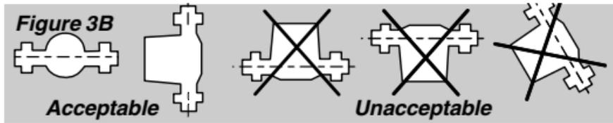
It is recommend that isolation valves be installed on each side of the pump. If possible, do not install elbows, branch tees, and similar fittings just before or after the pump. Provide support to the pump or adjacent plumbing to reduce thermal and mechanical stress on the pump.
