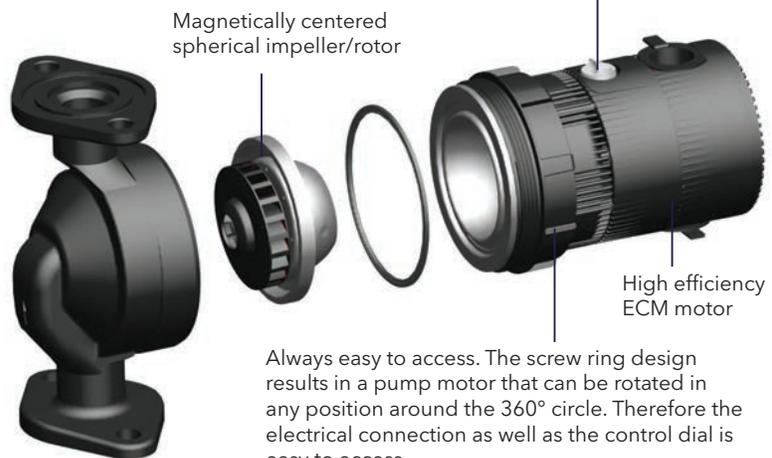
Magnetically centered spherical impeller/rotor
