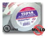
Printed 2 mil heavy duty, high strength aluminum foil coated with a specially formulated pressure sensitive acrylic adhesive system. Superior adhesion and conformance for use with fiberglass ductboard systems. Performance and materials guaranteed to meet or exceed UL181A-P quality standards; also meets the requirements of UL181B-FX, flexduct standard. Listed 89FL.
