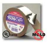
A 1.75 mil, high strength aluminum foil coated with an aggressive, high temperature acrylic adhesive system. Provides an excellent vapor seal on both fibrous and sheet metal ducts. Malleable foil also conforms well around corners and to irregular surfaces.
