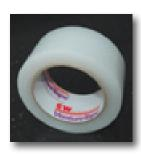
A 5 mil thick, strong and conformable polypropylene film tape coated with a very high shear, UV resistant acrylic adhesive system. Excellent holding properties and cold stick. Superior resistance to moisture, alkalis, oils, weathering and abrasion.
