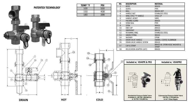
**Specifications:** Designed for residential or commercial use with potable water. This approved Webstone valve is actuated by a blowout proof stem and features an adjustable packing gland. Threaded ends comply with ANSI B1.20.1.
