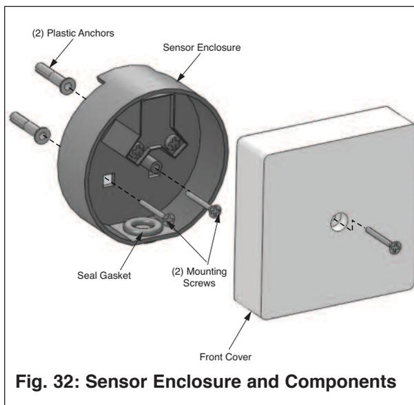
**Fig. 32: Sensor Enclosure and Components**
