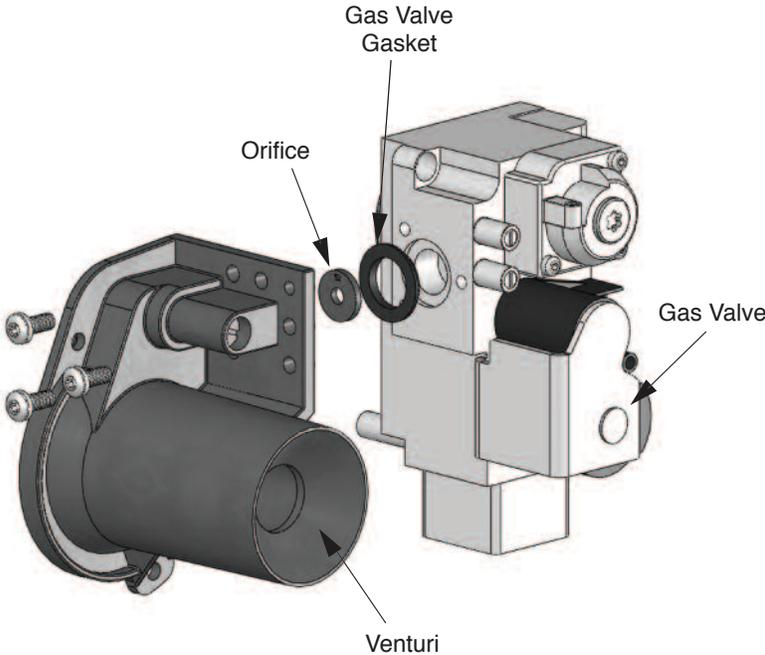
**Fig. 16: Gas Valve / Venturi Assembly - PRESTIGE Solo 60/175/250**
