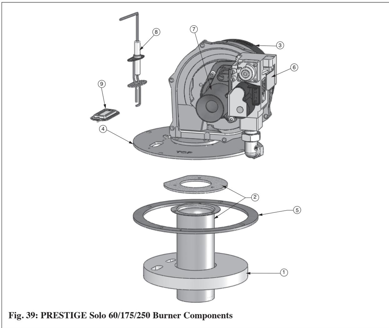
**Fig. 39: PRESTIGE Solo 60/175/250 Burner Components**
