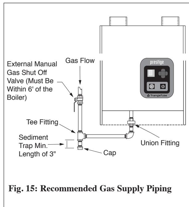
**Fig. 15: Recommended Gas Supply Piping**
