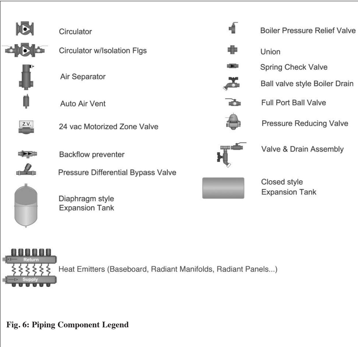
Fig. 6: Piping Component Legend
