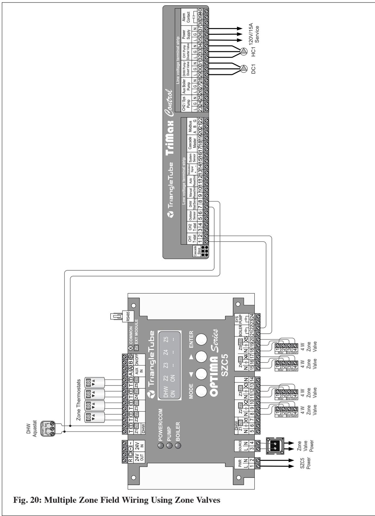
Fig. 20: Multiple Zone Field Wiring Using Zone Valves
