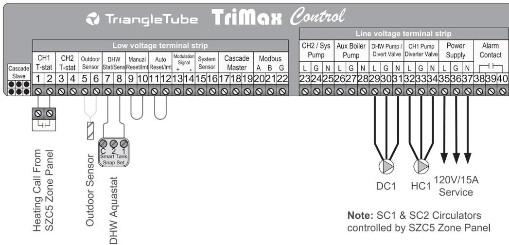
**Fig. 23: Prestige Wiring - Zoning with Zone Circulators**
