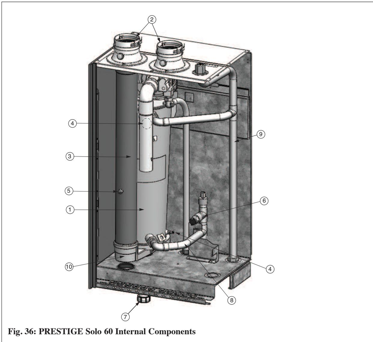
**Fig. 36: PRESTIGE Solo 60 Internal Components**
