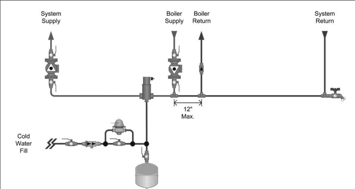
Fig. 7: Near Boiler Piping - Diaphragm Expansion Tank
