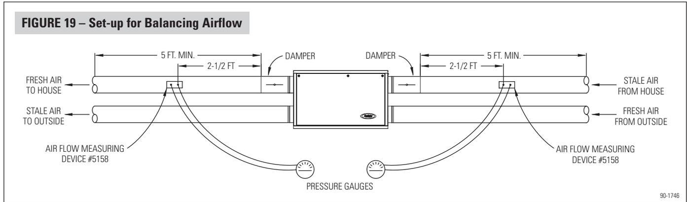
5. Verify the dampers are in the fully open position.
