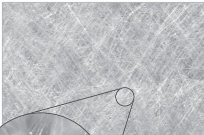
40x magnification shows the spun fiberglass skin of the StrataDensity<sup>®</sup> filter pad.
