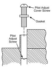
Figure 4. Pilot gas adjustment
