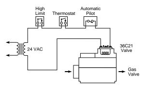
Figure 3. Wiring for 36C21 and 36C21A Models
