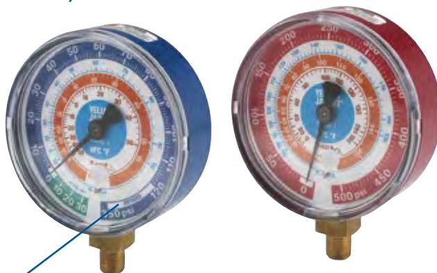
When a gauge has a **RETARD** zone, full scale is considered to be the last marked reading prior to entering the RETARD zone. For example, this gauge has a full scale reading of 120 psi. Gauge accuracy is not specified in the RETARD zone.
