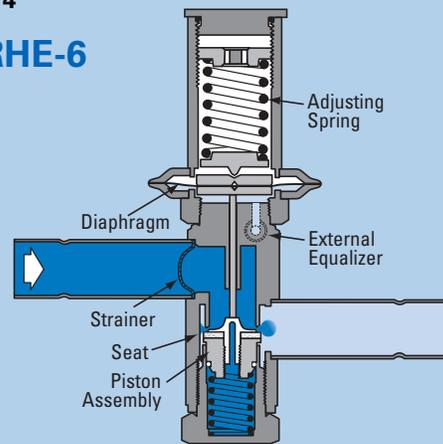
evaporator temperature change from closed position to rated opening. A 6°F change is considered normal for most applications and is the basis of our capacity ratings. Multipliers for other temperature changes are given in the Selection Procedures section.
