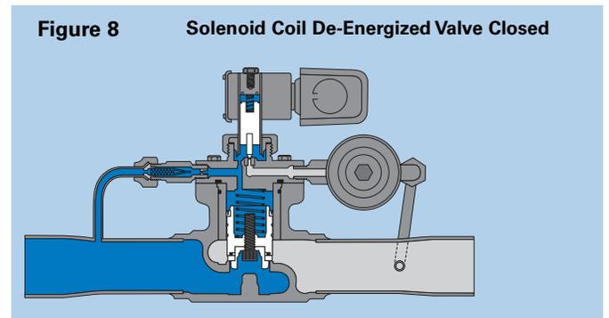
bleeds through the piston to the chamber above the piston. However, since the hot gas cannot bleed through the pilot valve, the pressure on top of the main piston (P3) increases, driving the piston down and closing the main port.
