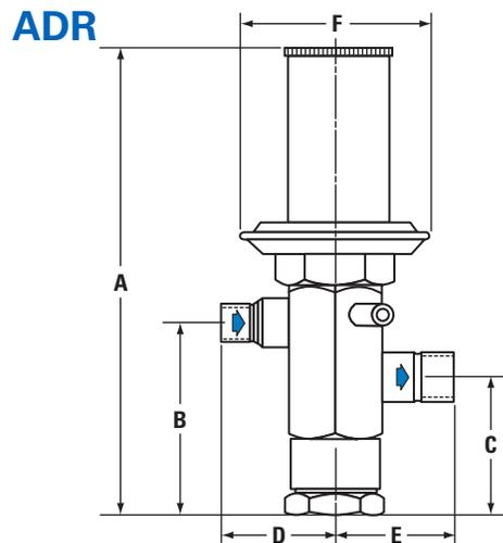
**PILOT OPERATED VALVES – SPECIFICATIONS and DIMENSIONS**
