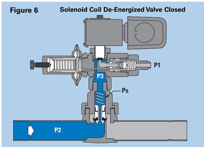
pilot valve, the pilot port modulates closed. This allows pressure to build on top of the main piston. As this pressure (P3) approaches the inlet pressure (P2), the force, combined with the force from the spring (P4), pushes the piston down, modulating the valve closed.
