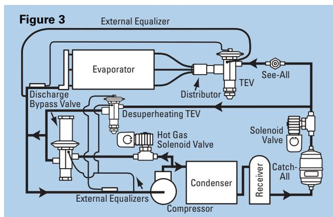
(Figures 1 and 3), require externally equalized valves, this model will be the most readily available one in the field. Therefore, it is suggested that in all cases, the externally equalized DBV be applied.
