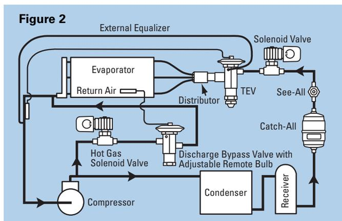
**Desuperheating Thermostatic Expansion Valve** – On those applications where the hot gas must be bypassed directly into the suction line downstream of the main expansion valve's bulb, an auxiliary thermostatic expansion valve — commonly called a desuperheating TEV or a liquid injection valve — is required.
