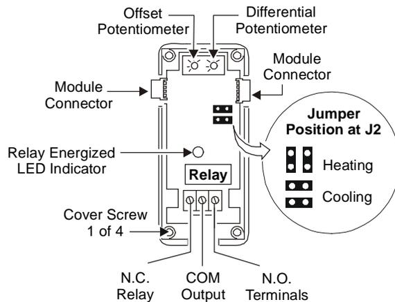
Figure 3: Interior View of S350A Stage Module
