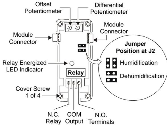
**Figure 4: Interior View of S351A Stage Module**
