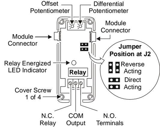
**Figure 5: Interior View of S352A Stage Module**
