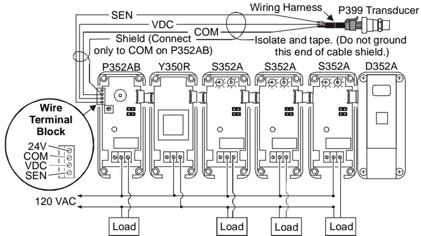
**Figure 11: Typical Multistage Pressure Control System Using 120 VAC Power Supply**
