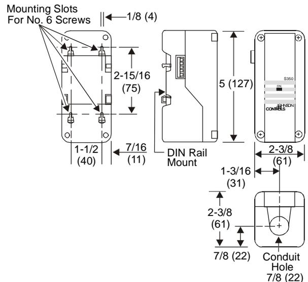
**Figure 2: System 350 Stage Module Dimensions, in. (mm)**
