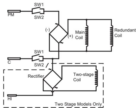
**WIRING DIAGRAM - HSI MODELS**
