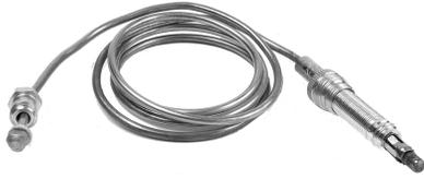
Thermocouples generate a thermoelectric current that senses a pilot flame on gas-fired heating systems. The pilot flame heats the tip of the thermocouple, producing a temperature differential between it and the base. This temperature difference generates a small amount of DC power, measured in millivolts.
