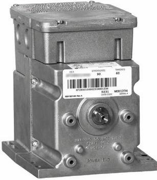
Series 41 and Series 81 Modutrol IV motors are 2-position (line- and low-voltage per motor control) spring-return motors. They are used to operate dampers or valves in applications where it is necessary or desirable to have the controlled element return to the starting position in the event of power failure or interruption.
