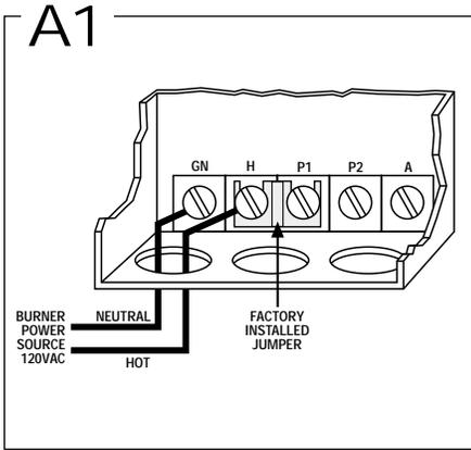
◀ **A1** Connect the hot lead of the input voltage (120 VAC, 60 HZ) to terminal H. Connect the neutral lead to terminal GN. 120 VAC, 60 HZ must be supplied to terminals H and GN for internal operation of the control.
