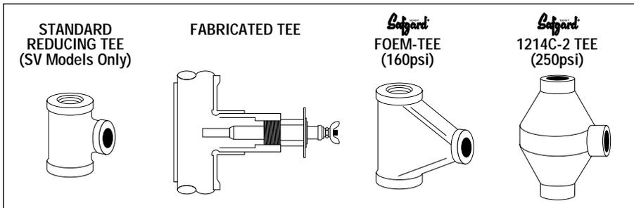
**TEE MOUNTING:** Model 170SV is equipped with the shorter EL1214-SV probe suitable for mounting in standard reducing tees. For other 170 Series controls, a fabricated tee can be used. Make sure that the tee drains thoroughly when water falls below it and that it conforms to the spacing requirements described in Step 3. Safgard tees are also available to accommodate all probe models (See page 4).
