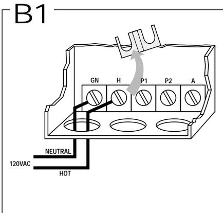
◀ **B1** **WARNING!** Remove the jumper between H and P1. Connect the hot lead of the input voltage (120 VAC, 60 HZ) to terminal H. Connect the neutral lead to terminal GN. 120 VAC, 60 HZ must be supplied to terminals H and GN for internal operation of the control.
