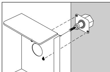
Slide keyhole slots over probe mounting screws and tighten screws (with either a 1/4" hex head driver or flat screwdriver).
