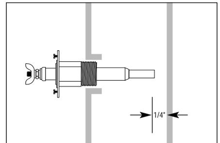
Check to insure 1/4" clearance from the probe to any surface within the boiler or tee. Apply pipe sealing compound to threads.
