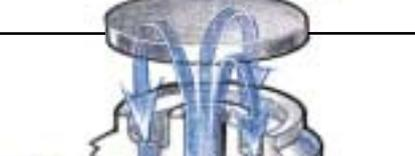
Hardened stainless steel disc with turbulence groove for rapid closing action.
