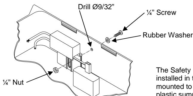
The Safety Float Switch may be installed in the drip pan or it may be mounted to the side of the molded plastic sump tank, as shown.
