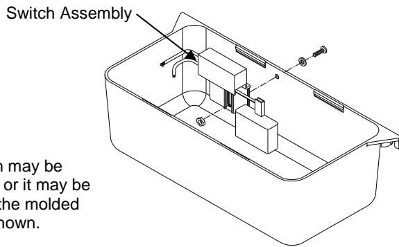
**WARNING:** Risk of electric shock, the remote Safety Float Switch is not submersible and should be connected only to an N.E.C. Class II circuit of not more than 30 volts.
