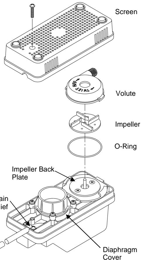
**CAUTION:** The cord of this pump contains a small "Breather Tube". This tube is necessary for the proper operation of the pressure switch. Do not allow this tube to become blocked.
