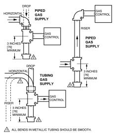
CAUTION: SHUT OFF THE MAIN GAS SUPPLY BEFORE REMOVING END CAP TO PREVENT GAS FROM FILLING THE WORK AREA. TEST FOR GAS LEAKAGE WHEN INSTALLATION IS COMPLETE.
