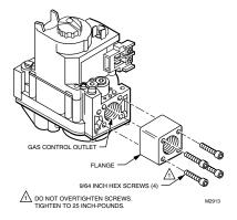
form on the control after completing the installation includes leak testing the adapters and screws. If you use a wrench on the gas control after flanges are installed, use the wrench only on the flange, not on the control.
