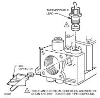
Fig. 8—Wiring connections.
