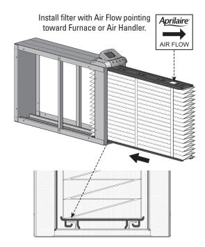
Align filter in top and bottom rails and slide into place. Reinstall door.
