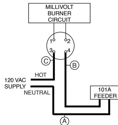
**For Model 101A-24 Feeder and Model 67G with millivolt burner circuit**
