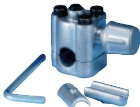
SUPCO's "Bullet® Piercing Valve" utilizes the same type of gasket found under the head plate of most air conditioning compressors. When installed, the gasket actually compresses the copper tubing .020" creating a permanent, leakproof seal that will withstand any pressure and temperature for the life of the unit.
