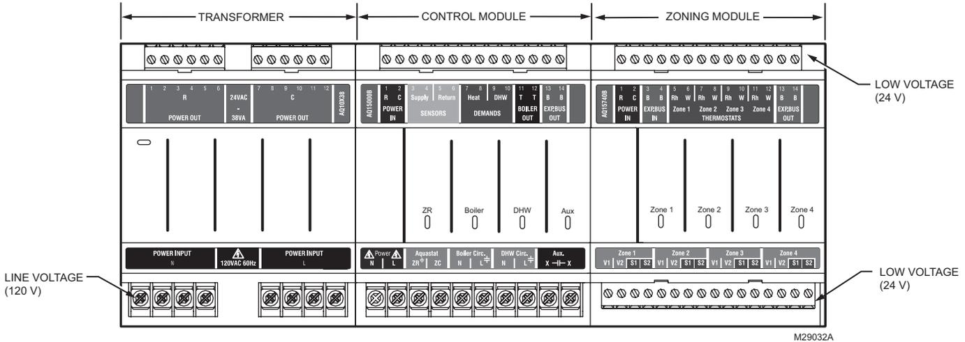
Fig. 1. AQ250 Control Panel layout (AQ25044B shown).
