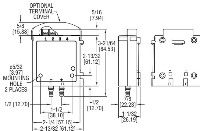
The Series 616KD One-Touch® Differential Pressure Transmitter senses the pressure of air and compatible gases and sends a standard 4 to 20 mA or optional voltage output signal. A wide range of models are available factory calibrated to specific ranges. A single push button properly adjusts both zero and span. New enclosure enables the 616KD-A/B to be mounted on a 35 mm DIN rail either via its side or back DIN rail clips.
