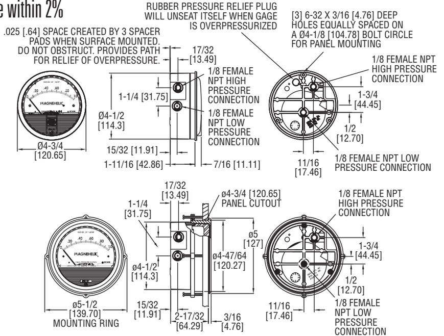
Select the **SERIES 2000** Magnehelic® Gage for high accuracy--guaranteed within 2% of full scale--and for the wide choice of 81 models available to suit your needs precisely. Using Dwyer's simple, frictionless Magnehelic® gage movement, it quickly indicates low air or non-corrosive gas pressures--either positive, negative (vacuum) or differential. The design resists shock, vibration and over-pressures.
