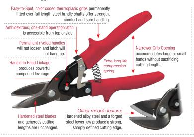
The Max2000 Double Cut Snip employs a best of all worlds close tolerance design for consistent performance. A curved cutting edge on the center jaw reduces cutting force required and large relief grinds on all jaws minimize drag. The double cut blades feed smoothly, cut cleanly without surface distortion, and easily navigate metal seams encountered in round metal duct and stove pipe. A self-starting point on center jaw makes short work of
