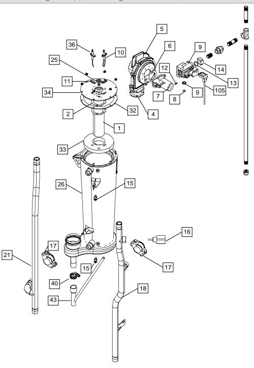
Figure 17-1(b) Tft Cabinet, Vent and Air-inlet Parts (Tft60-110 Illustrated)
