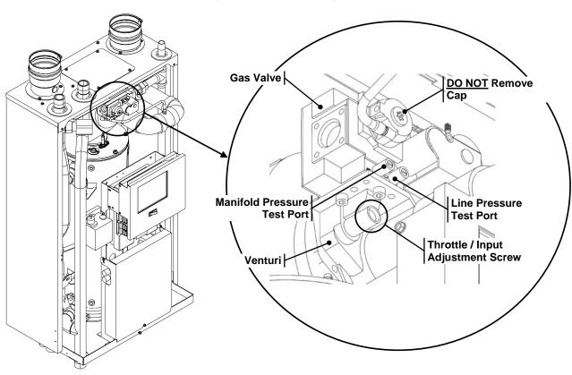
Figure 9-2 Tft300-399 Gas Valve and Venturi Assembly
