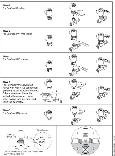
If the actuator will be used with a cord length of >3m and max. 23m, the protection of the cord/wire (overload, short circuit and mechanical stress) should be assured by a circuit breaker (6A/characteristic "B") and should be installed in a protection tube or comparable means.
