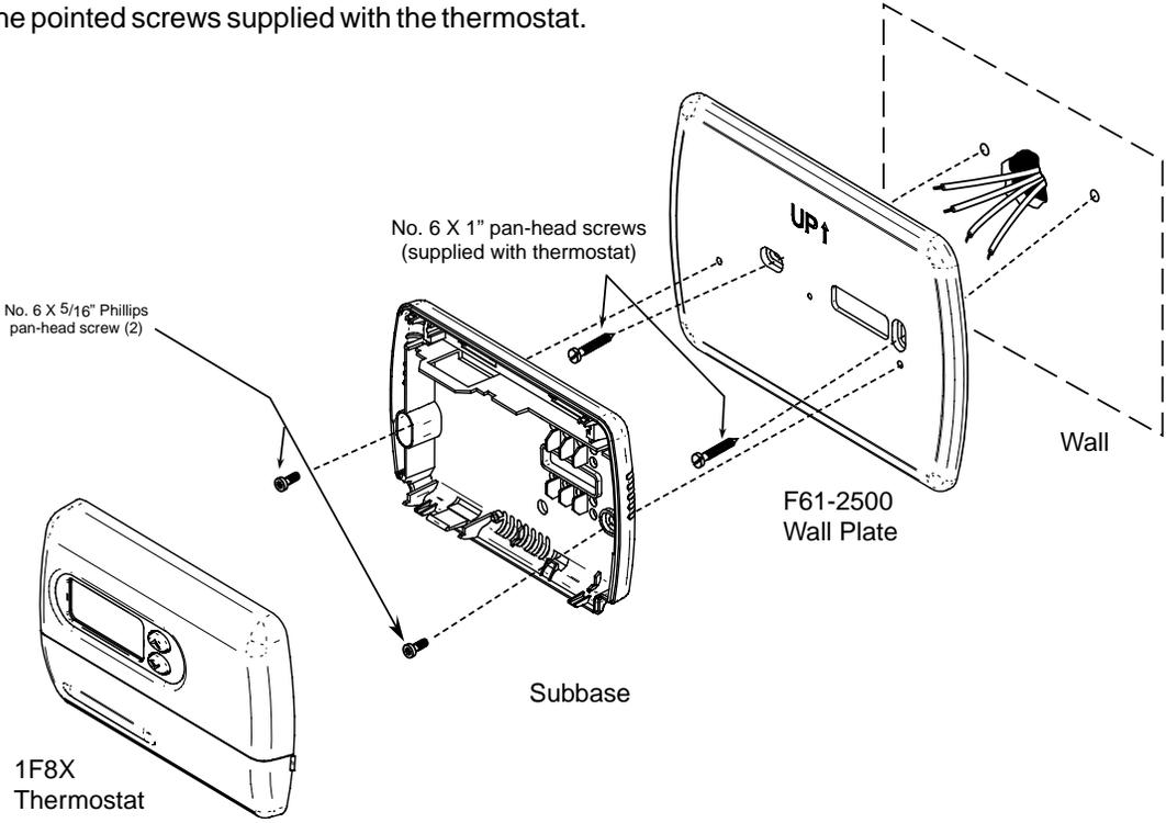
**Figure 3. Mounting 1F8X digital thermostat to wall**
