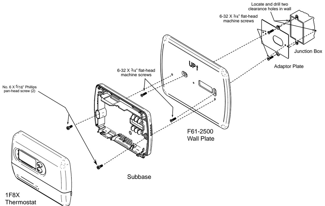
Figure 2. Mounting 1F8X digital thermostat to vertical junction box
