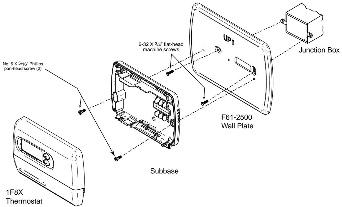
Figure 1. Mounting 1F8X digital thermostat to horizontal junction box
