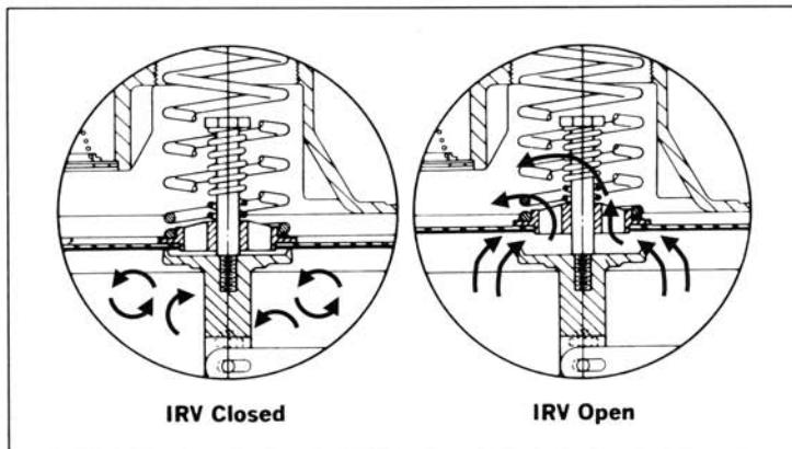
**Caution:** Note that an IRV, like any other relief valve, must be sized carefully. If the curves indicate that outlet pressure can exceed the maximum safe limit it is essential to provide an additional relief valve carefully sized to handle the difference.
