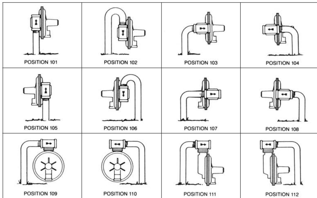
**NOTE:** If desired position is not shown use diagrams at right as guides to specify vent, diaphragm case, and body arrangement.
