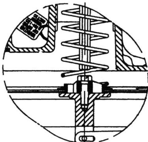
A travel stop is located in the 243-12-1 and the 243-12-4 to provide overpressurization protection.
