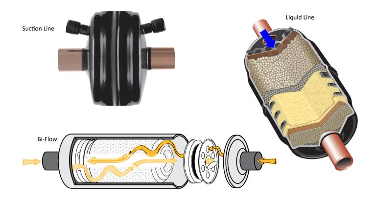
All Parker Steel Liquid Line Filter-Driers are rated at 600 PSI working pressure.
