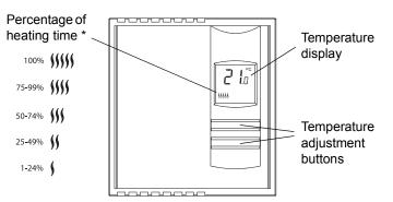
\* The thermostat displays the percentage of heating time required to maintain the desired temperature. For example, *ss* is displayed when heating is activated 40 percent of the time.
