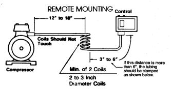
The capillary between the vibration coils and the control body should be secured to a stationary member when that distance exceeds 6 inches.
