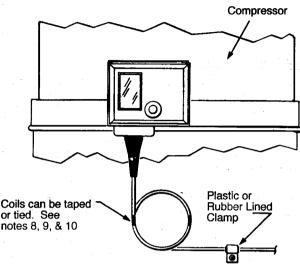
7. When the control body is mounted remote from the compressor and the pressure connections are on the compressor, vibration coils must be used between the compressor and the mounted con-trol. The coils should not touch. A section of rubber pipe insulation inserted into the vibration coils and secured with silicone adhesive will keep the coils separated, yet allow them to absorb vibration.
