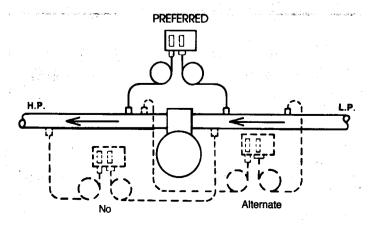
6. When the control is mounted directly on the compressor, the capillary must be secured to the compressor so that everything moves together. If the capillary or control is shaking or vibrating against the compressor vibration, work-hardening of the capillary may occur, leading to eventual failure.
