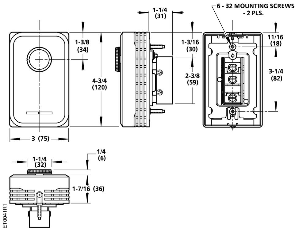
Figure 7. Dimensions of 134-1084, 134-1085 and 134-1086 Thermostats.
