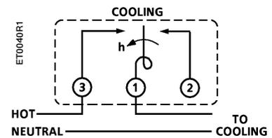
Typical cooling application for 134-1084, and 134-1085 thermostats.
