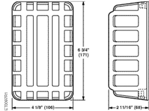
Figure 6. Dimensions of the 134-117 Thermostat Guard.
