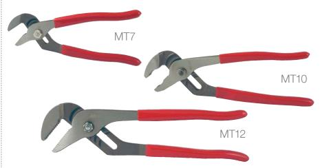
Tongue and groove joints hold jaws securely in selected position and take strain off bolt. Teeth are designed to give maximum grip on any round, square or hex shaped object. Long cushion grip handles give powerful leverage with gentle angled spread for easy one hand operation. Thin design permits access to confined spaces where conventional pipe wrenches won't go. Tempered steel halves offer long dependable service.
