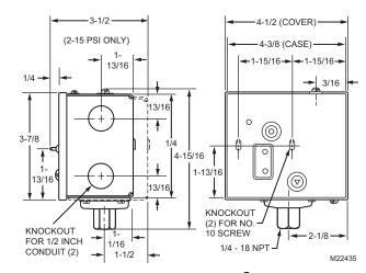
Fig. 1. L4079A,B,W PressureTrol<sup>®</sup> Limit Control dimensions in inches.
