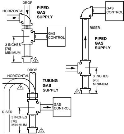
3. Thread pipe the amount shown in Table 4 for insertion into the gas control or flange. *Do not thread pipe too far.* Valve distortion or malfunction can result when the pipe is inserted too deeply into the gas control.
