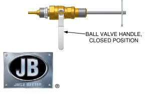
4. You may now unthread BY HAND (release counter-clockwise) the knurled back body from the Core Removal Tool and remove the shaft/body assembly.
