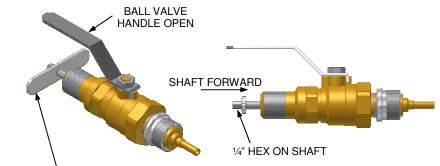
NOTE: DO NOT USE THIS HANDLE TO TORQUE THE CORES. USE A TORQUE GUN OR TORQUE WRENCH OVER THE  $1\!\!\!/4''$  HEX IN THE SHAFT.
