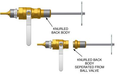
NOTE: While Core is removed, processing can be performed through the Seat and Core Removal Tool. Do not remove from the Seat until the Core is torqued back into the Seat.
