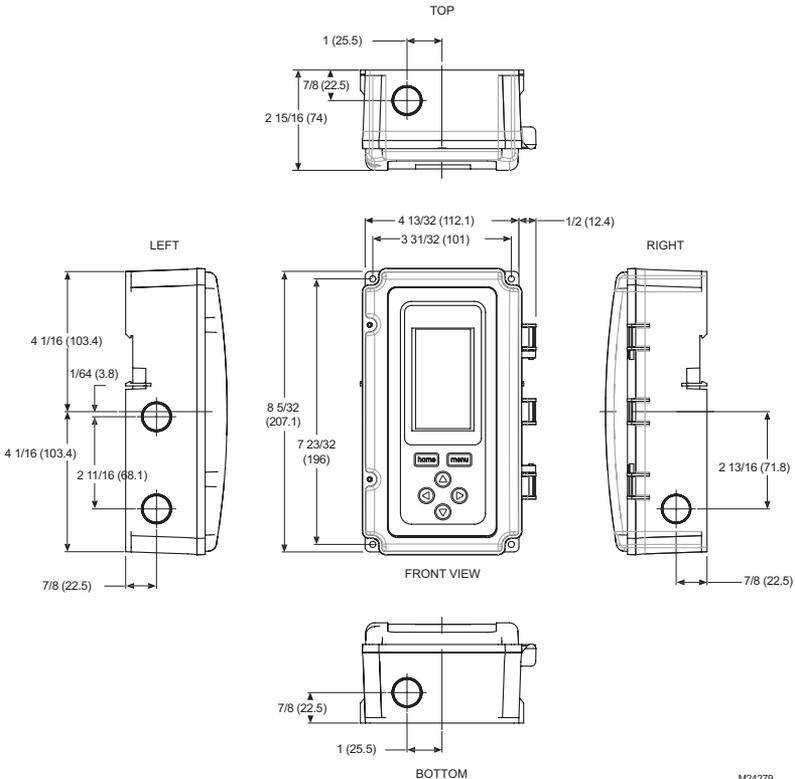
Fig. 1. T775A/B/M Dimensions in inches (mm).
