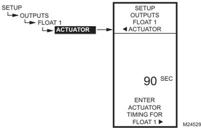
Fig. 65. Setup - Outputs - Floating Relay - Actuator.
