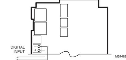
**Fig. 14. Wiring for Digital Input (Dry Contact).**
