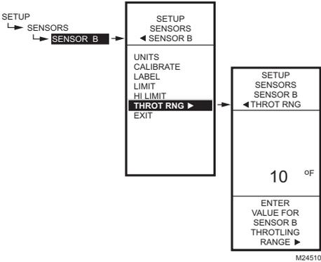
Fig. 44. Setup - Sensors - Sensor B - Throttling Range.
