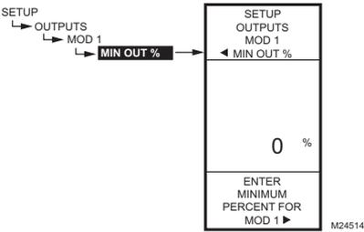
Fig. 48. Setup - Outputs - Mod Out - Minimum Output Percentage.
