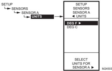
Fig. 37. Setup - Sensors - Sensor A - Units.
