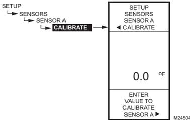
Fig. 38. Setup - Sensors - Sensor A - Calibrate.
