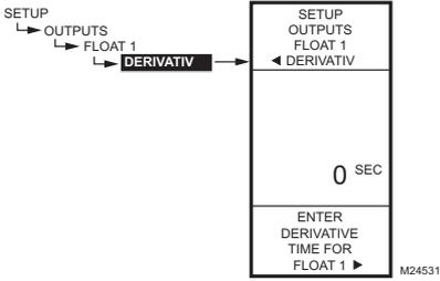
Fig. 67. Setup - Outputs - Floating Relay - Derivative.
