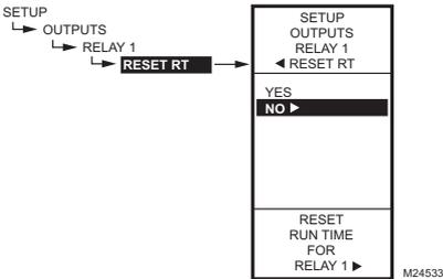
Fig. 69. Setup - Outputs - Relay - Reset Runtime.
