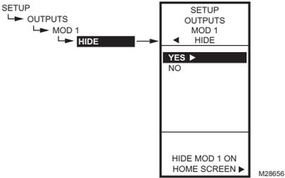
Fig. 52. Setup - Outputs - Mod 1/2 - Hide.
