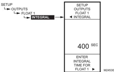
Fig. 66. Setup - Outputs - Floating Relay - Integral.
