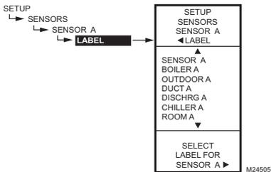
Fig. 39. Setup - Sensors - Sensor A - Label.
