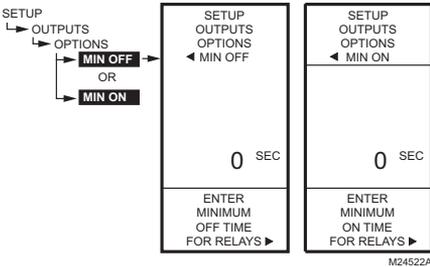
Fig. 57. Setup - Outputs - Options - Min Off/On Time.
