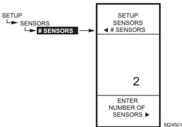
Fig. 35. Setup - Sensors - Number of Sensors.
