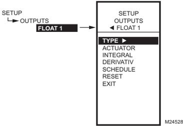
Fig. 64. Setup - Outputs - Floating Relay - Menu.
