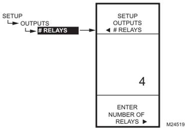
Fig. 54. Setup - Outputs - Number of Relays.
