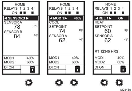
Fig. 23. LCD Display - Home Screen Displaying Sensors, Active Relays, and Mod Outputs.
