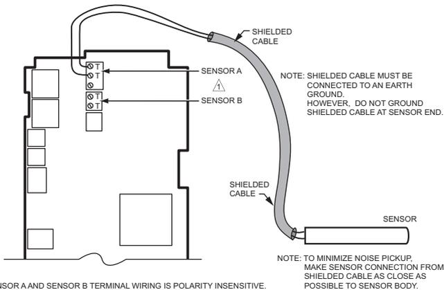
**Fig. 4. Sensor Wiring — Showing Shielded Cable Connection to Sensor A.**
