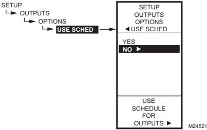
Fig. 56. Setup - Outputs - Options - Schedule.
