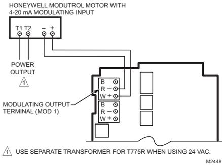
⚠ USE SEPARATE TRANSFORMER FOR T775R WHEN USING 24 VAC.
