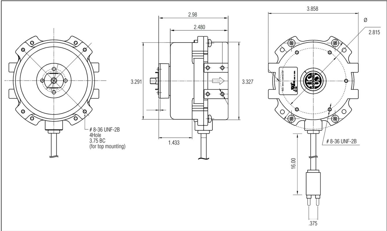
Kit 58 available to be used when replacing rectangular, 51 frame, EC motors to adjust for fan position or when a flat mounting surface is needed
